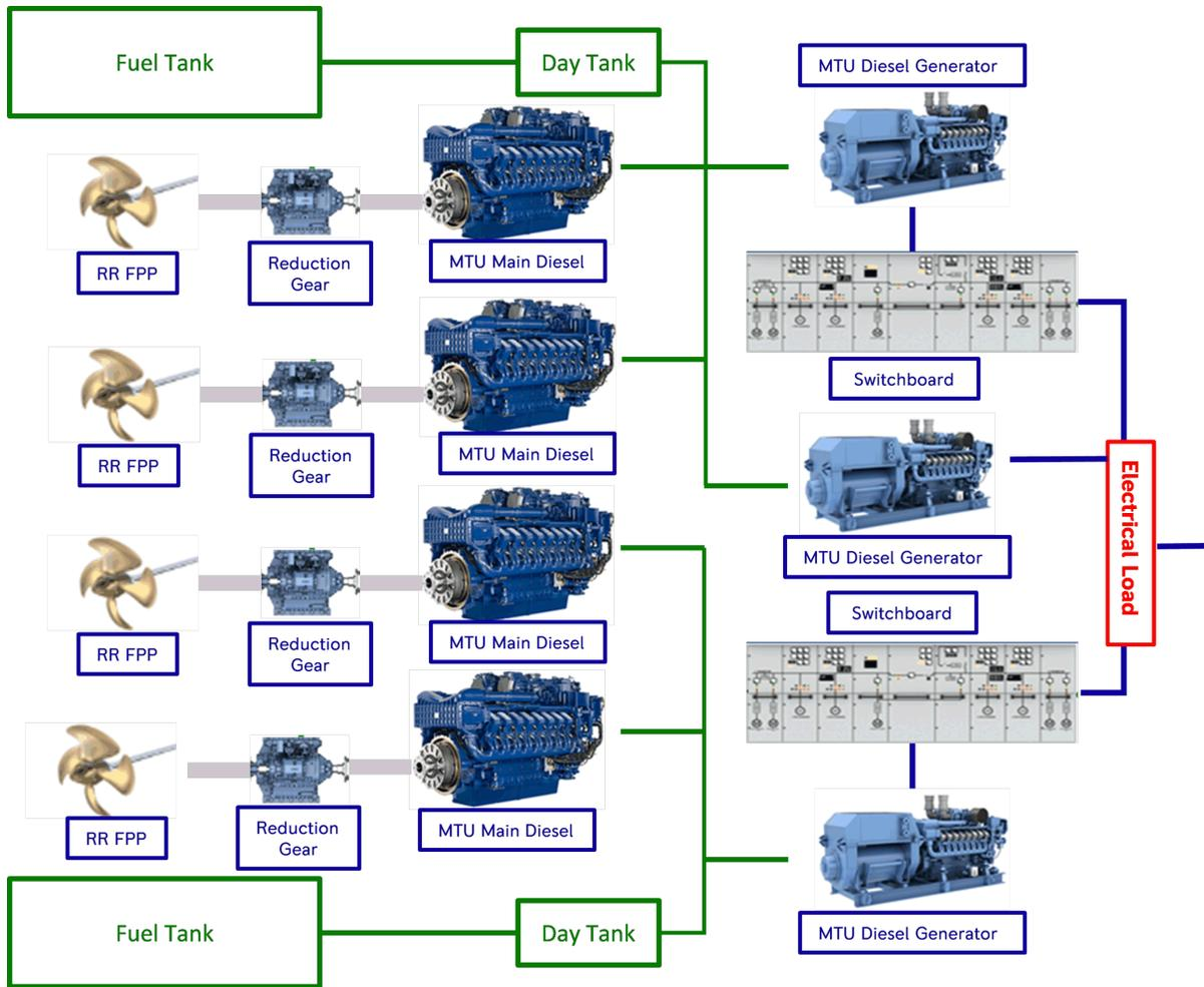
**Figure 2. Conceptual USV Power and Propulsion System**
